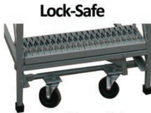
Casters retract with weight on the first step. Pull the handle to release lock.
